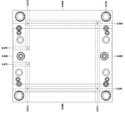
All C-TLU'S can be modified in length and width to accommodate cams or waterlines. Leader Pin locations can be moved. 2 more Leader Pins and Bushings can be added for an additional cost. All ear-plate and ejector locations will stay the same. All guided ejection and return pins options are available. (see Page 22)
